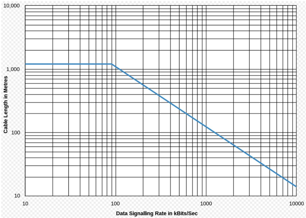
**Ensure you are using twisted pair wire like Local Area Network (LAN) with value of CAT 5E or higher. If you are finding errors, ensure you have grounded both ends. The unused pairs should be used for ground connections. In my case, no ground wire was used/needed.**
